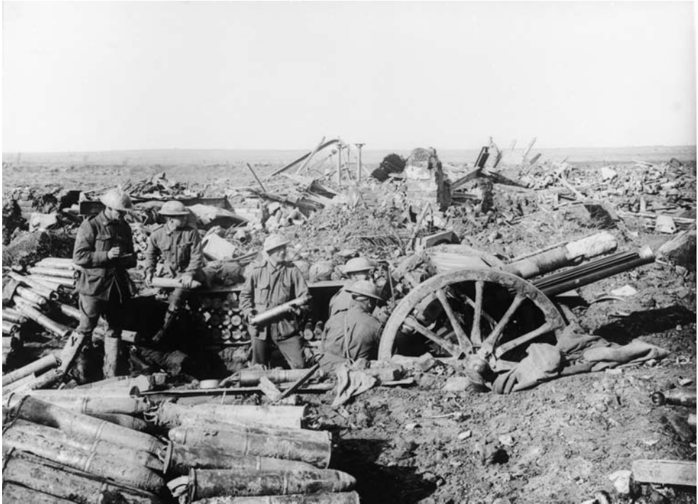
AWM E01209. An 18-pounder gun of the Australian Field Artillery dug in among the ruins of an old factory.
